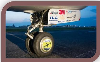
**Prototype electric wheel tug system**
